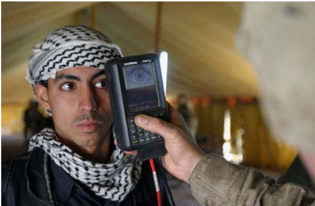
The Biometric Analysis Tracking System uses thumbprints and facial and retinal scans to identify foreign persons of interest to human intelligence and counterintelligence personnel.
