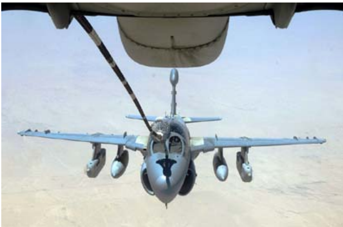
Air refueling is a key part of most air interdiction operations and extends the range, payload, and endurance of air interdiction assets, thereby increasing their effectiveness.
